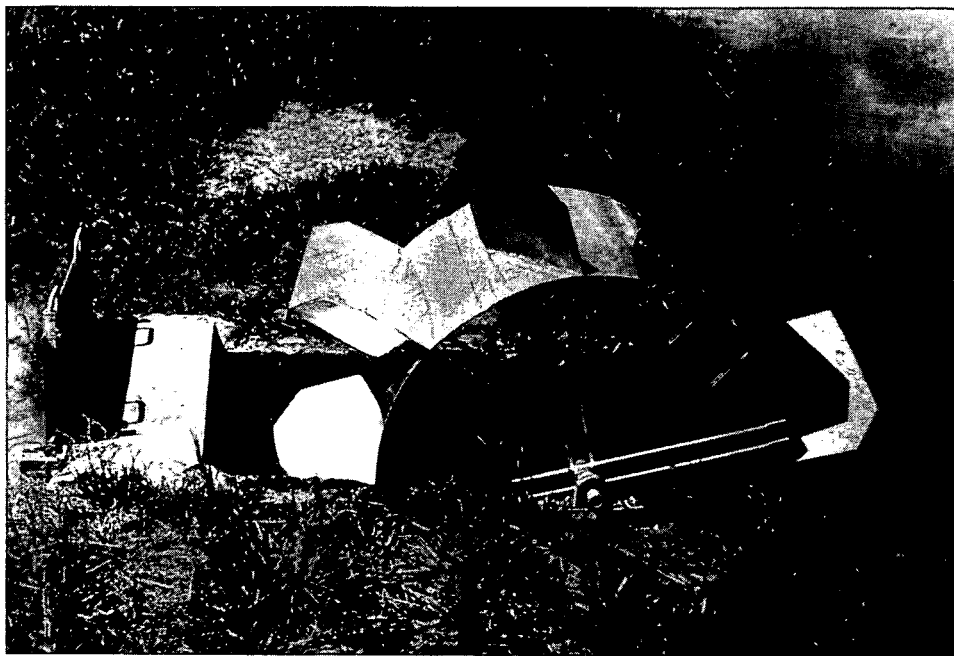
Photo 4 One of the vanes was painted red to check the revolutions counter and required gate openings
